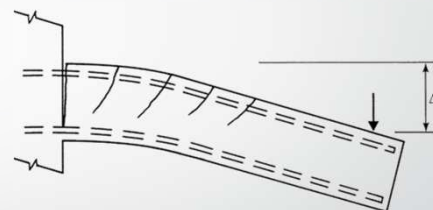
(a) Cracks due to load acting downward
